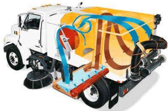
The Elgin Crosswind recirculating vacuum sweeper efficiently cleans our City streets and provides two primary benefits to the City. The more obvious benefit is the collection and removal of paper, leaves, and other visible debris that collect in gutters and on the streets. In addition to being unsightly, this debris can block catch basins and other storm
